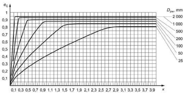
Fig. 5.7 Fouling factor for a circulating oil lubrication system with on-line filtration \beta_6 = 200
