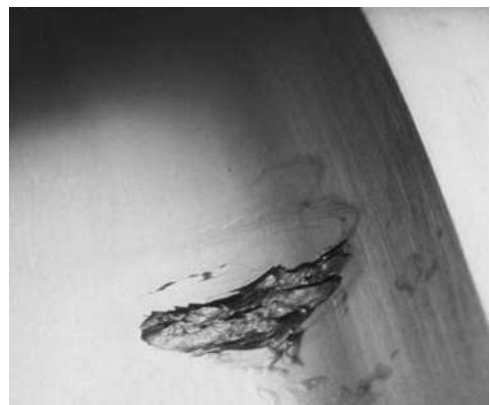
Fig. 5.2 Photo-illustration of fatigue damage on the raceway
