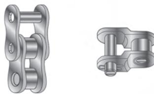
The main components of a roller-type transmission chain are shaped side plates, roller bearing pins and rollers. The distance between the centre of two pins determines the chains pitch.
