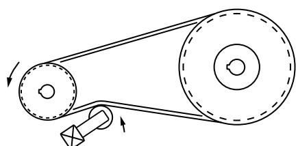
**V-Belt Tensioner - Inner Grooved Pulleys**
